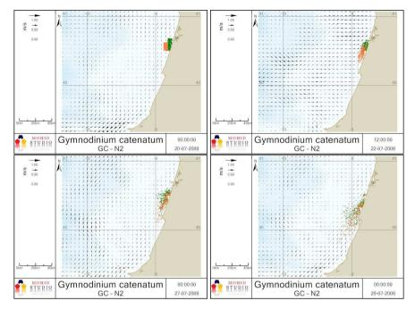
**Figure 3.** Transport of the *G*. catenatum bloom with an origin in the Vagueira area (scenario GC-N2). Particles with distinct colors are used to differentiate the path of particles with different origins.
