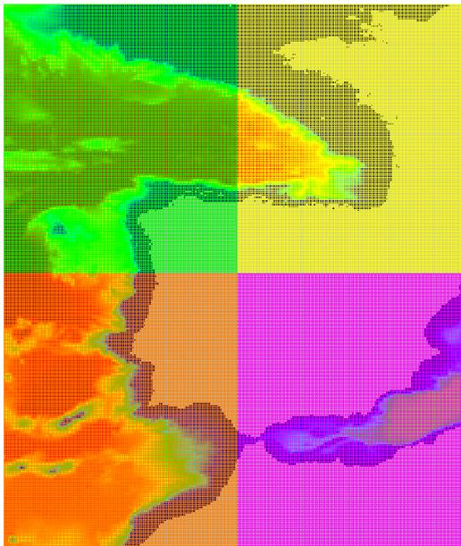
*Figure 4 : Possible domain decomposition specified by the user.*
