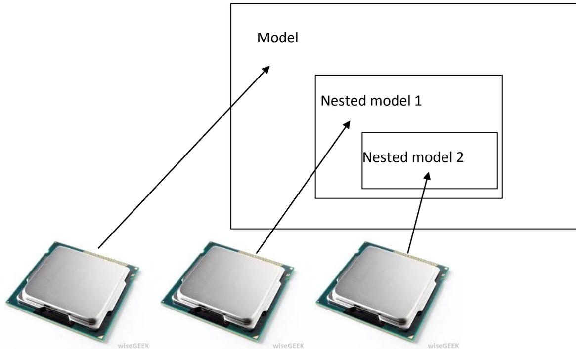
Figure 1 : Diagram showing the workload distribution for the MOHID parallelization methodology “one model – one process”.
