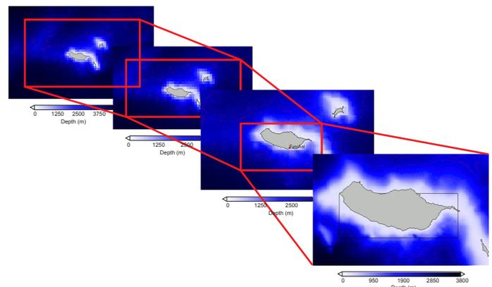
Figure 2. System of nested grids used for simulating the hydrodynamics and ecology of the Madeira Island.
